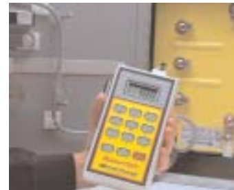
The MasterTEST connects to the ISB to perform real-time system testing of the EGPE2.
