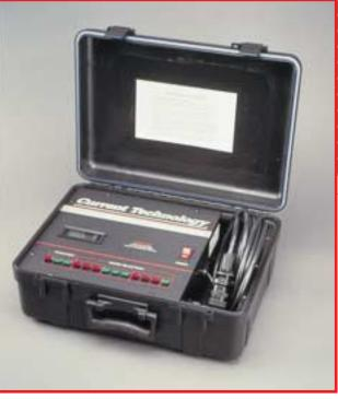
All Current Technology MasterPLAN suppression filter systems are shipped with a DTS-2 Diagnostic Signature Card listing factory-established benchmark testing parameters. By routinely testing and monitoring Current Technology suppression filter systems, recording each reading and comparing any variances, end users are assured of maximum suppression filter system performance.
