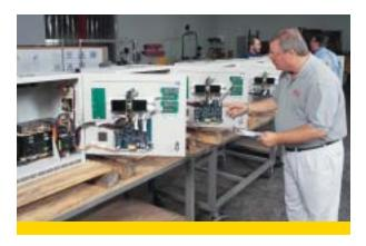
Simulator for on-site product testing. The accepted standard for sustained product life evaluation, the KeyTek ECAT permits on-site testing with amperages of up to 10,000 amps and voltages as high as 20,000 volts. SELect suppression filter systems are subjected to strenuous testing and inspection by diligent quality assurance pro fessionals before leaving the factory, and every unit is shipped with a Diagnostic Signature Card listing factory-established benchmark performance values.\*
