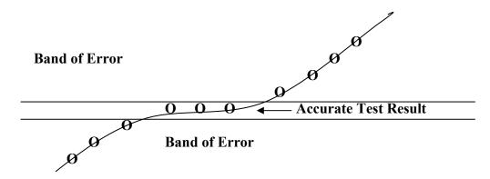
A highly trained, experienced technician will be able to determine the resistance of the ground rod after a number of readings are taken by moving the intermediate electrode away from and then closer to the rod under test. The most remote electrode must remain in the same position for the results to be accurate.
