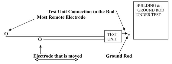
The most remote electrode must be placed a minimum of 5 times the distance of the length of the ground rod being tested. It is preferable the most remote electrode be placed a distance equal to 10 times the length of the rod under test. During the test the neutral must not be connected to the ground rod. The neutral / ground bond must be disconnected as the current flow on the neutral will invalidate the test results and not all the test instrument to provide an accurate reading.
