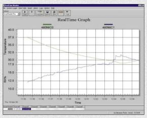
Run the ACR RealTime Graphing Software while TrendReader® or POWERWATCH® Software for Windows® is running to view the realtime data in a graphical format. Realtime graphing allows you to visually detect potential problems before they turn into disasters. Since ACR Data Loggers accumulate historical data, you can still look back and analyze logged information.
