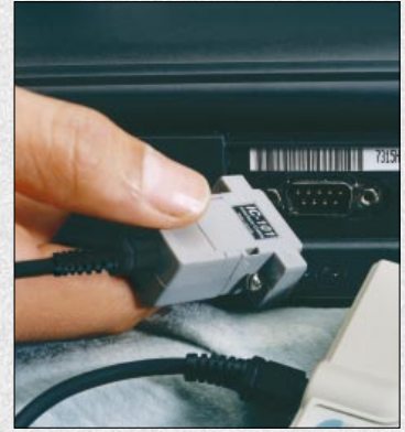
How the IC-101 connects between the SmartReader Plus Data Logger and the PC serial port.
