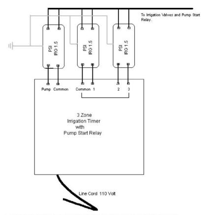
\* Note: To gain maximum efficency of PSI Isolated Loop Protector all electrical components (distribution panel, isolated loop protectors, pump motor and well casing) must be bonded together. This will prevent "back door" damage due to a ground loop (imbalance in ground potential).
